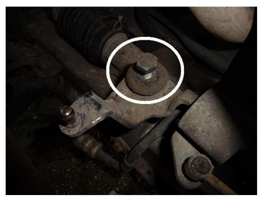
Unscrew the bolt which holds the OEM shifter. (use 16mm spanner) Remove shifter arm and undo it from all components.
