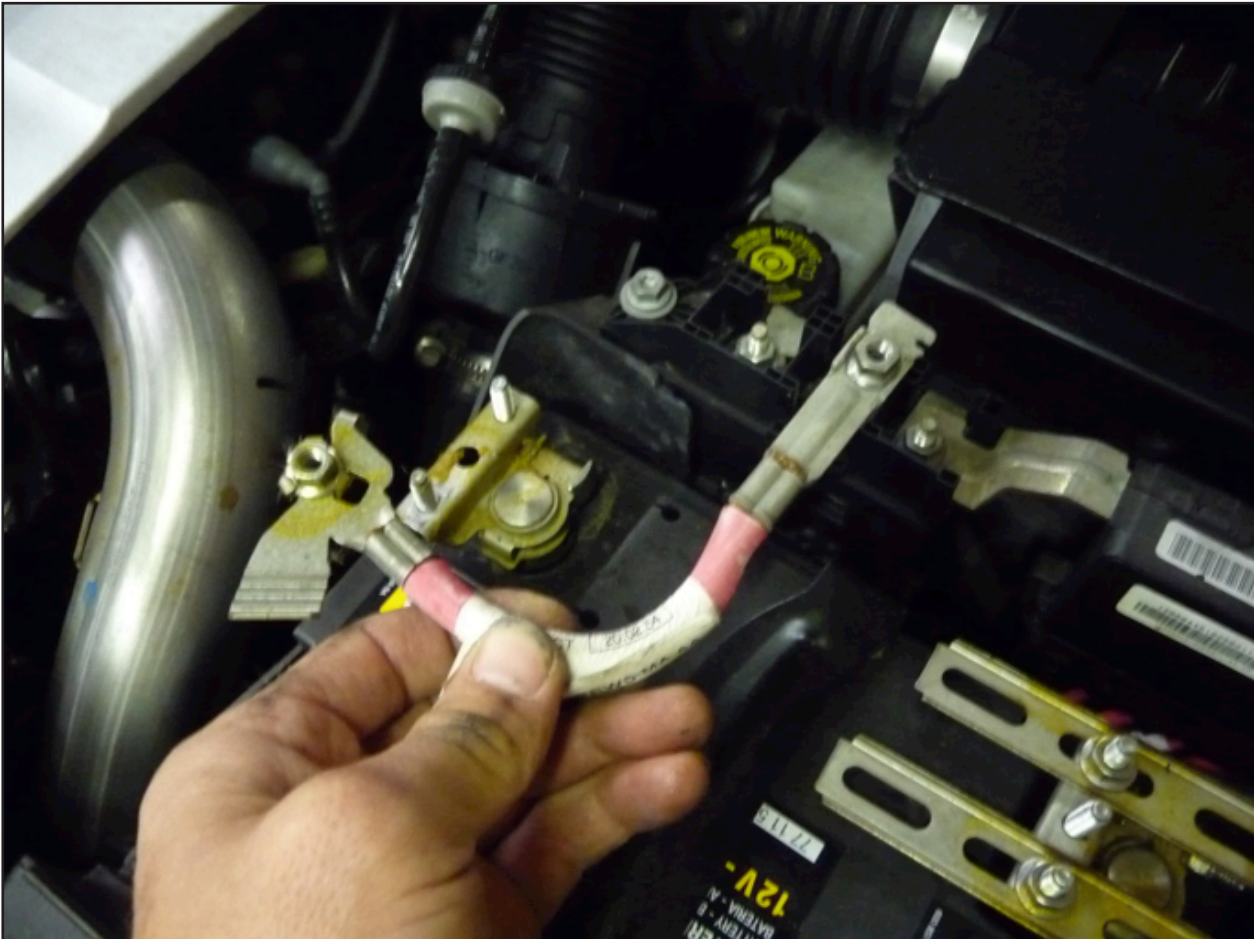
Remove battery cover and 12V plus cable (2x M6)
