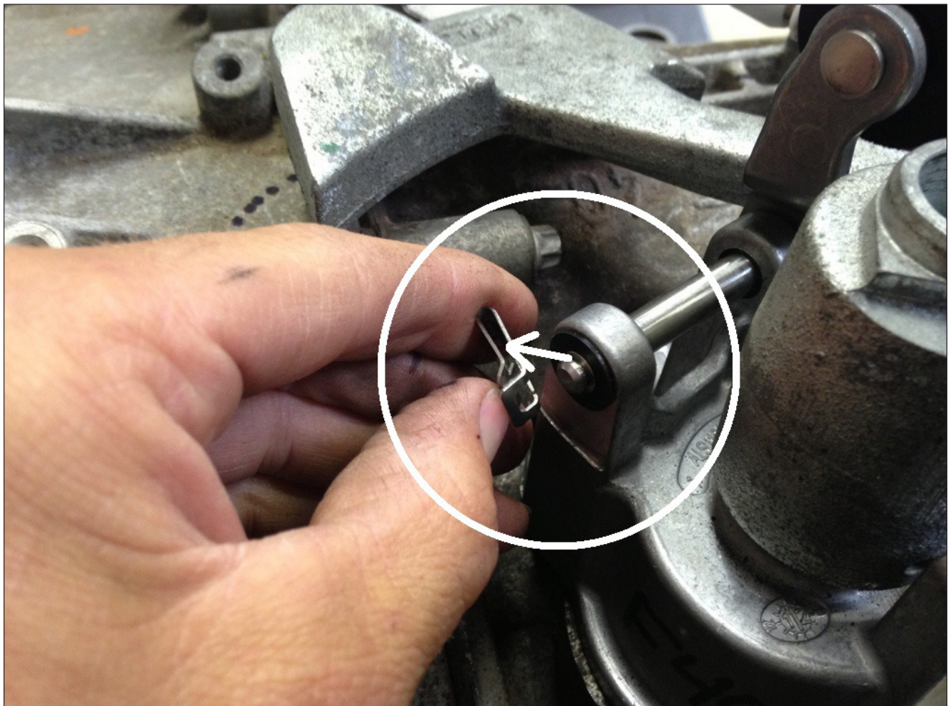
Remove metal clip and replace it with our special secure ring (included).
