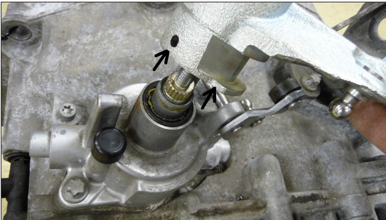
Remove old leaver and put new short shift in place.
