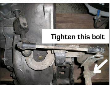
Keep the gear leaver in the neutral position agianst the left side and keep it in this position. (Line of the first and second gear). Ask someone to keep the leaver in this position and tighten the bolt.
